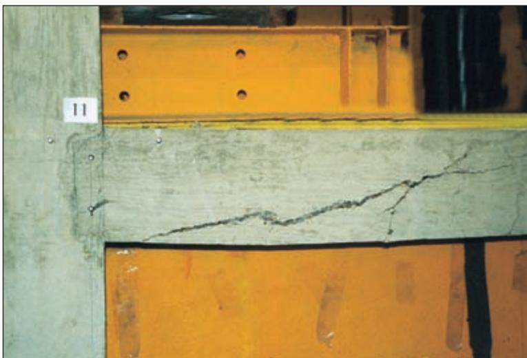
Post-test cracking after loading slab 800mm from wall/slab junction. Kwikastrip continuity reinforcement was incorporated top and bottom of slab.
