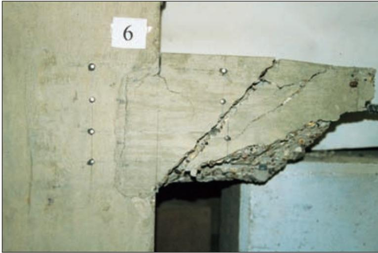
Post-test cracking after loading slab 300mm from wall/slab junction. Kwikastrip continuity reinforcement was incorporated in top of slab only.
