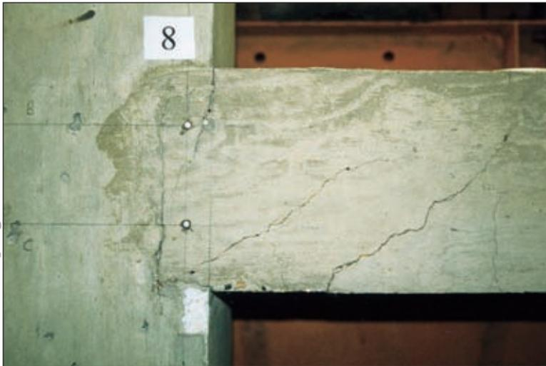
Test configuration as (6) above, except continuous polystyrene section cast into joint soffit/interface to simulate poor compaction of concrete in wall.
