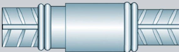
3 Finished joint tightened with a wrench until no further movement between sections
