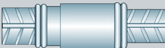
3 Finished joint tightened with a wrench until no further movement between sections
