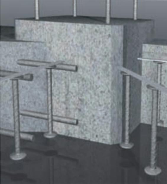
The code contains various detailing requirements, particularly in relation to the spacing of the elements of shear reinforcement and various limits on for example the concrete compressive strength, which may be taken into account in design against punching.
