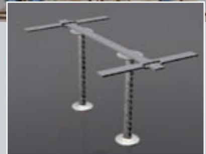
**Figure 3 - Rail Spacing Device**
