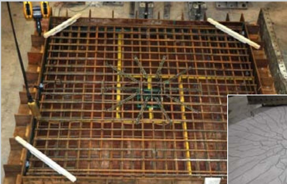
Figure 3 - LinkStudPSR Testing
